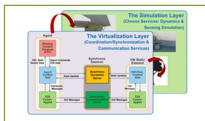
Synchrono multi-agent simulation framework allows multiple vehicles to be simulated in the same environment and scenario. Each vehicle can leverage Chrono for high-fidelity physics and sensor simulation.
